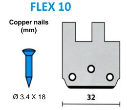
Type-Flex hinged fasteners are produced in galvanised iron and non-magnetic stainless steel which are fastened by means of copper nails whose round section allows an excellent tensile stress resistance performance. They can be applied in the workshop and on the construction site by using a hammer and cutting pliers.
